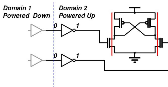
Fig 2. Crossbar currents in differential signaling due to incorrect powering scheme.
