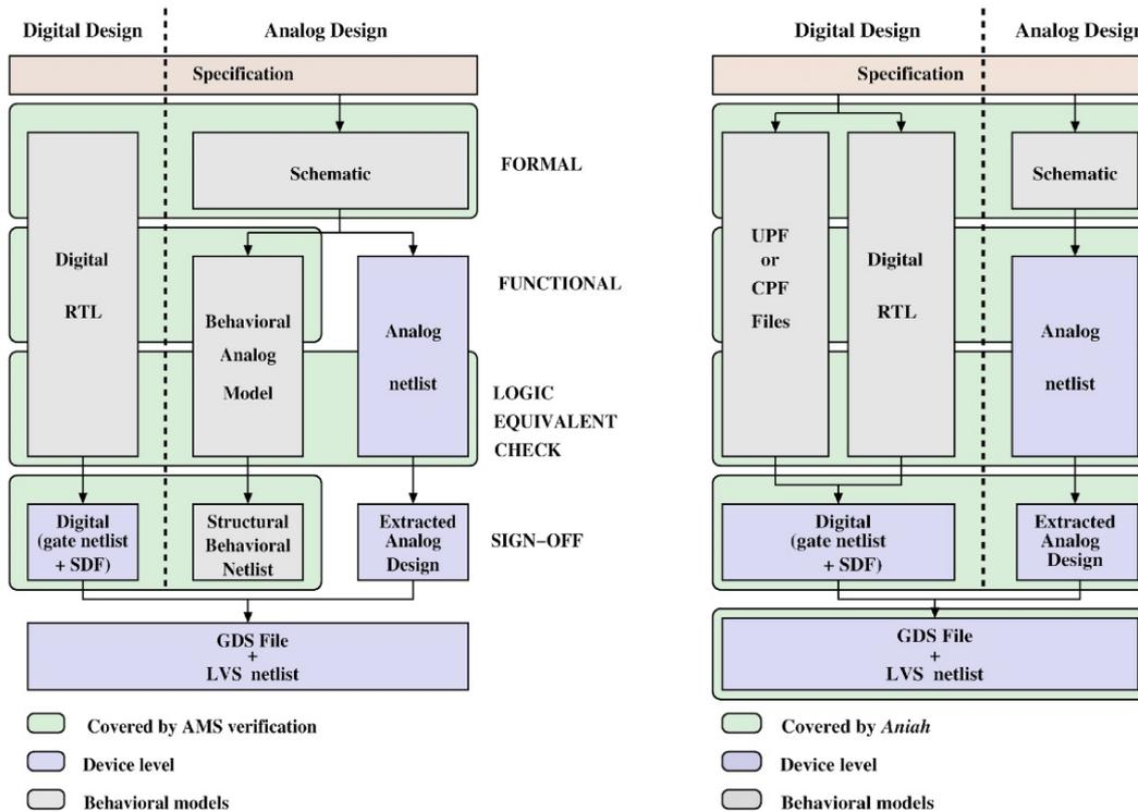
Fig 4. (a) Analog Mixed Signal Verification Methodology.
