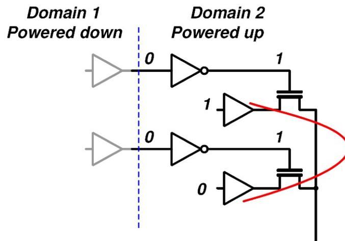
Fig 1. Crossbar current caused by an improper powering scheme at the domain boundary.
