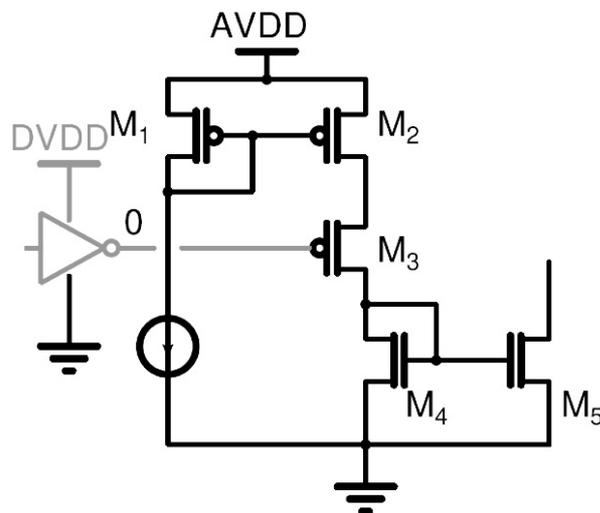
Fig 3. An analog block might be powered even after bias has been disabled.
